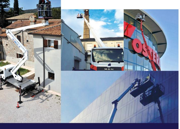
TM20 20.00m Max Lift Capacity: 230kg
